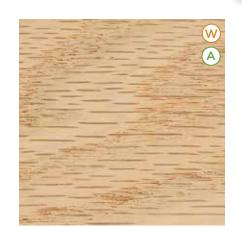
Red Oak is known for its strength and stability and has a prominent open grain. Oak ranges in color from white to yellow to reddish brown. Small pin knots and minor mineral streaking are present. Graining may vary from closely knit to a sweeping arch pattern.
