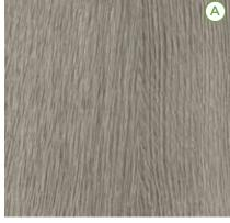
**Thermo Structured Surface (TSS)** has the look of real wood veneer with greater color uniformity, durability and ease of maintenance. TSS is a thermally hardened surface created when 100% pure melamine resins, along with special phenolics are heated and pressurized. TSS door styles have color coordinating PVC edge band and are available in both horizontal and vertical grain. Grain pattern and color tones are not bookmatched.
